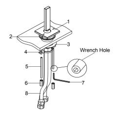
Attach the hoses(8) to water supplies. The hose with blue mark connects to cold water. The hose with red mark connects to hot water.
