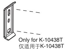
2. Drill the marked mounting holes with a 6mm bit and insert wall plugs.
