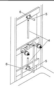
Install G1/2" pipes(4) and ells(6) to the bath and shower outlets. Secure the bath and shower pipes to the support.
