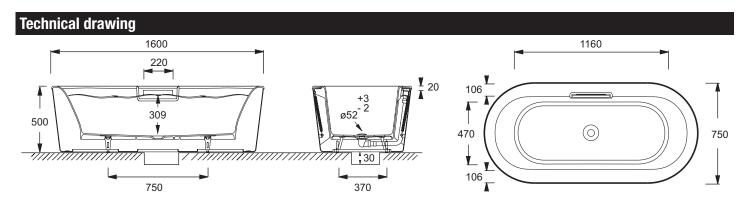
Product Specification: Freestanding bath 160 x 75 cm. 6D062. Collection: VOLUTE. Dimensions: 160 x 75. Weight: 135 kg. Material: Cast iron. Installation: Floor-standing. Volume: 170/100. Shape: Oval. Incl. factory-assembled reinforced acrylic panel and built-in waste 6D064. Trap and connection kit E75307. To install waste, lay trench 3 cm deep in the floor or build platform..
