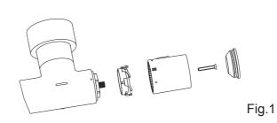
Mark sure the reference mark is aligned with number 38 before your action. Remove the handle kit.
