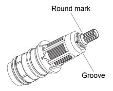
**NOTE:** Do not turn the cartridge when reinstall it. If you turned it without carefully, you should adjust it and be sure that the round mark is correctly in line with the groove, or readjust as per the steps of verification and setting.
