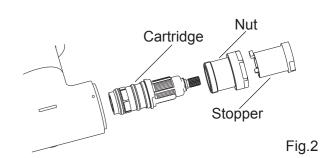
Unscrew the nut and stopper. Removing the cartridge cautiously. Clean the thermostatic cartridge by soaking it in warm vinegar.
