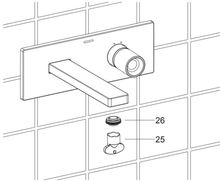
Ensure that all coupling nuts are tight. Ensure that the handle is in the off position.
