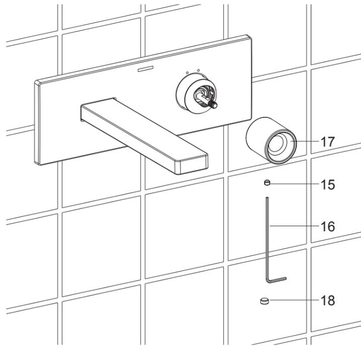
Valve closed, and loosen the screw(15) on the handle with 2.5mm hex wrench (16).
