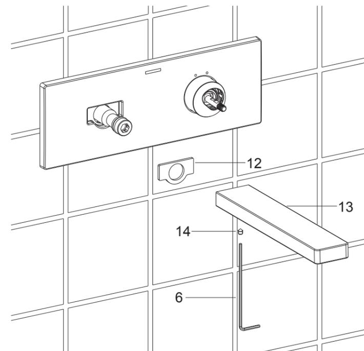
Slide the washer(12) into the groove on the faceplate kit.
