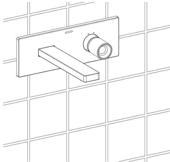
The illustration shown is the correct position of the spout and handles when the installation is complete.
