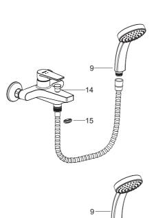
Ensure that all coupling nuts are tightened.
