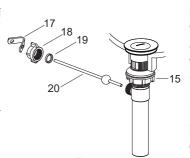
Remove the retaining nut(18). Fit the plastic washer(19) and retaining nut onto the ball lever(20). Insert the ball lever assembly into the drain lever hole and through the stopper hole. Tighten the retaining nut.
