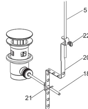
According to the lift rod length, bend the link(20). Connect the link onto the lever(18) with "V" clip(21). Slide the lift rod(5) into the hole on link. Push the lever down to the open position. Tighten thumb screw(22).
