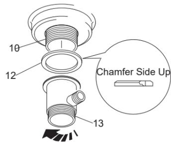
Install the seal(12), secure and tighten the drain body(13) to the waste by hand.
