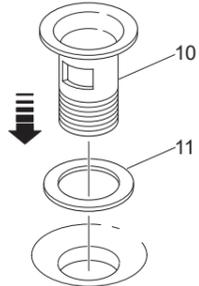
Install the waste(10) with foam ring(11) into the drain hole.
