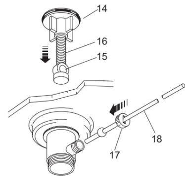
Adjust the drain body to enable the ball lever(18) and lift rod(5) to engage.
