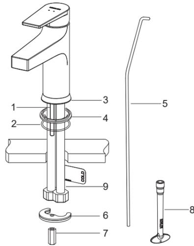
Install the mounting stud(1) onto the bottom(3) of the faucet. Insert lift rod(5) to the rear hole of the body. Put O-ring(2) onto the base(4). Install the base into the underside groove of faucet body through the hoses(9), lift rod and mounting stud.
