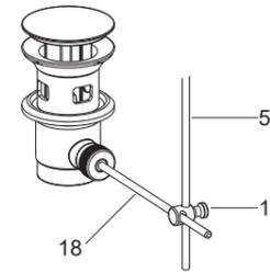
Attach the connector(19) onto the ball lever(18) and lift rod(5). Tighten the connector retaining screw with a suitable screwdriver.
