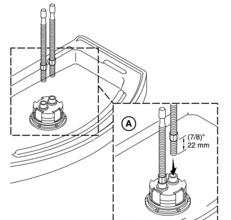
**16A.** Install the tank lid and test the length of the push button rods. When the rods are correctly adjusted, the button will have a firm and consistent push.
