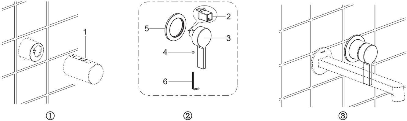
As figure 1 shown, remove and discard the protector(1) after completing the finished wall. Turn off the valve.
