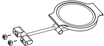
6. Insert the pins of the adapter into the power outlet at the bottom of the light base. Insert the adapter to the socket. Switch on and it is ready for use.
