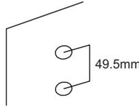
3. Drill 5mm holes at the points marked in step 2 with a 5mm drill. Apply silicon sealant to the drilled holes and insert the wall plugs.
