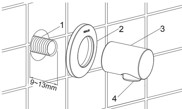
To perform installation, installer must provide G1/2" nipple(1) to the pipe so it extends 9~13mm beyond the finished wall. Apply tape or thread sealant to the nipple threads.
