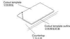
Trace the outline of the cutout template on the countertop with a pencil at the desired installation location. Use a pencil in the kitchen work surface to mark the desired location of the sink installation. Trace the outline of the cutout template on the countertop.
