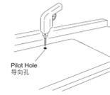
Cut along the outline to cut out the opening in the countertop along the marked outline. Cut out the sink opening.
