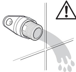
Turn on the water supply and flush the pipework.
