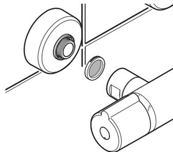
Assemble the bar valve with a sealing washer / filter in each inlet and attach to the wall bracket.
