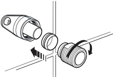
Install the olives and the connectors. Tighten finger tight and then another 1/4 to 1/2 turn.
