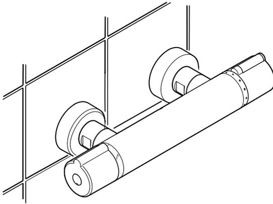
Tighten the connections, turn on the water supply and check for leaks.
