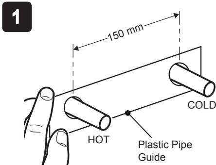
Fit the plastic pipe guide over the inlet pipes. Level the pipe guide and secure to the wall to hold in position. **Leave the guide in place and finish the wall.**
