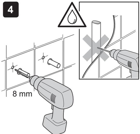
Drill the fixing holes using an 8 mm diameter drill.
