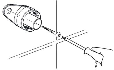
Install the fixing screws (supplied) and tighten.
