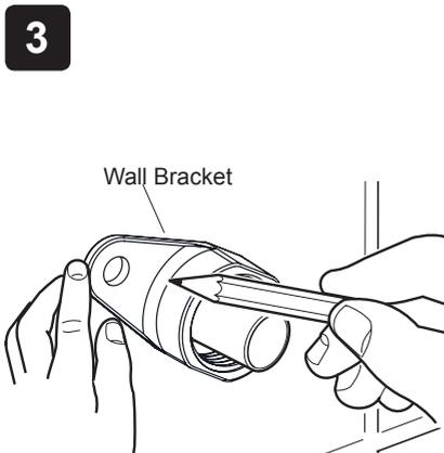
Hold the wall bracket in position and mark the position of the fixing holes.
