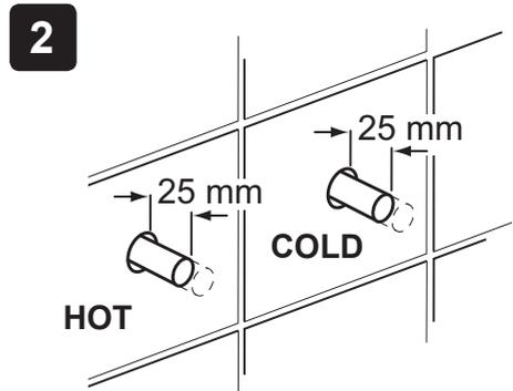
Make sure that the pipework has been installed correctly and that it protrudes 25 mm from the finished wall surface.
