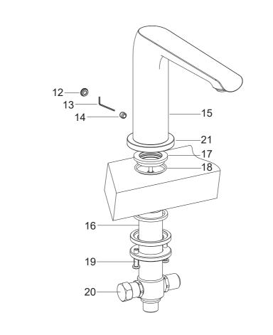
Tighten the nut(17) with the o-ring onto the diverter kit, and keep it against the bath tub. Position the diverter kit so that the nut(20) is on the left. Tighten the screws(19) to secure the diverter kit.
