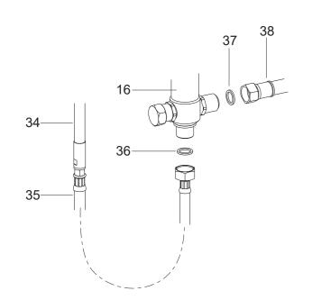
Put the washer(36) into the nut of the hose(35). Connect the connection hose to the diverter kit(16).
