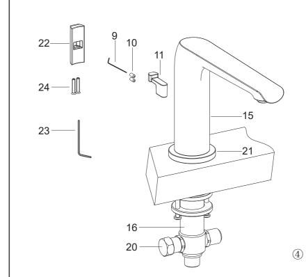
Install the connector(11) to the diverter kit
