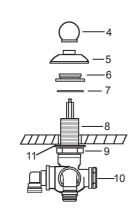
Remove the knob(4), escutcheon(5), base nut(6), rubber washer(7) from the shank(8) of the body assembly in turn.
