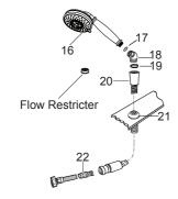
Slide the hose(20) through the hose guide(21), and attach to the hose(22).
