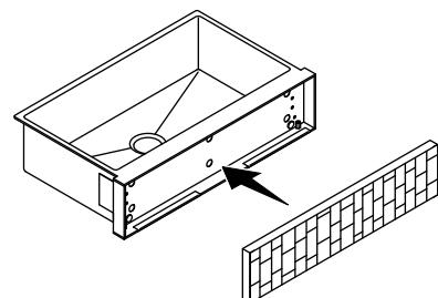
**8 Slide a bolt with lock washer through one of the holes in the pocket. The bolt must engage the threads at the top of the pocket. Handtighten.**
