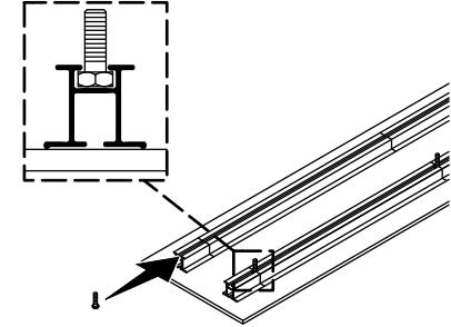
**3 Align the bolts with the marks on the rails.**
