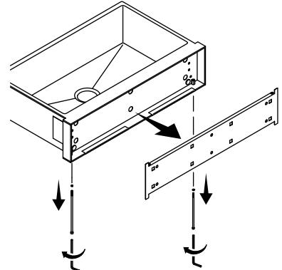
**2 Lay the insert face down and slide three bolts into each metal rail.**
