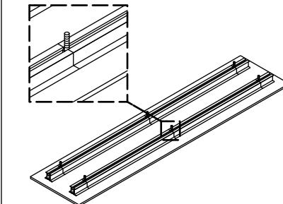
**4 Center the carrier over the insert so the bolts go through the round holes.**
