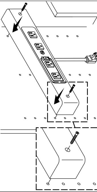
**2** Electric Shelf Installation: Insert the four brackets into the peg holes. Align the shelf notches over the brackets. Snap the shelf in place.
