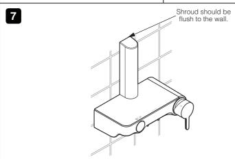
Slide the shroud over the clamp plate and assemble with the body.
