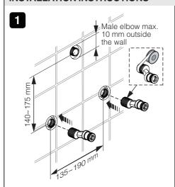
Apply the thread sealant tape on the threads to avoid leakage.
