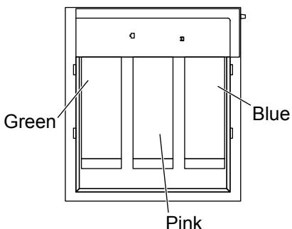
**NOTE:** The filter cartridges require conditioning prior to use to remove air and carbon particles. The filter cartridges will be arranged differently for cartridge conditioning than when the cartridges are in use.
