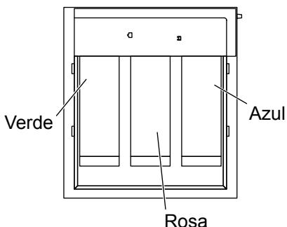
**NOTA:** The filter cartridges require conditioning prior to use to remove air and carbon particles. The filter cartridges will be arranged differently for cartridge conditioning than when the cartridges are in use.
