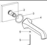
Insert the washer(3) into the bottom groove of the spout(4).
