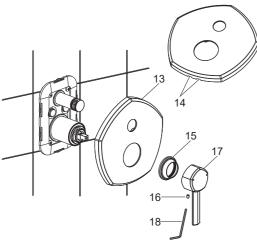
Slide the faceplate(13) onto the valve with slots(14) downwards. Push it until it is against the wall.
