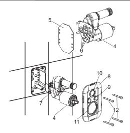
Remove the protection(5) on the valve kit(4). **NOTE:** Don't drop the O-rings(6).
