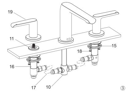
Secure the side bodies(16) by tightening screws(18) with screwdriver.
