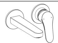
When the installation is completed, the correct position of the spout and handle with the valve closed is shown in the figure.
