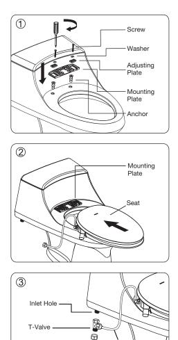
\ Hose • Secure the mounting plate over the inserts of the toilet bowl with the screws and the washers provided. Tighten the screws with a screwdriver.
