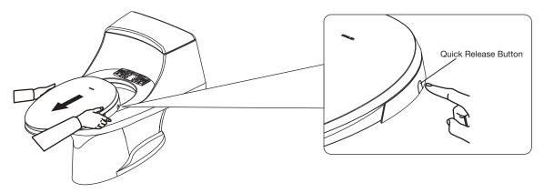
• Push the quick release button and slide the bidet seat out of the mounting plate.
