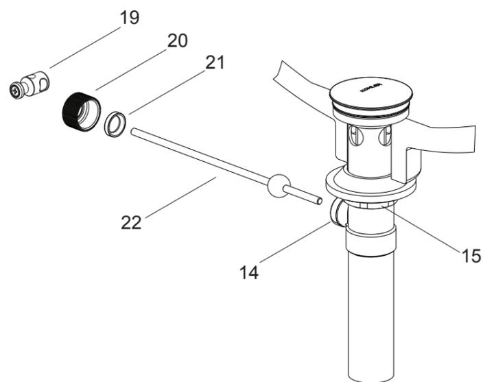
Remove the latch(19) and retaining nut(20). Fit the plastic washer(21) and retaining nut onto the ball lever(22). Insert the ball lever assembly into the drain lever hole and through the stopper hole. Tighten the retaining nut.
