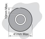
Before installation, installer must provide G1/2" nipple (1). The nipple should extend 11mm beyond the finished wall. Make sure the gap between the nipple and finished wall is not more than 10mm. The hole's maximum diameter is 41mm in the wall.
