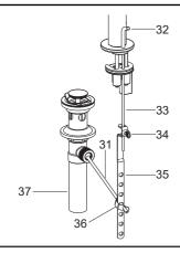
**NOTE**: Do not reposition the drain after the locknut is tightened, or you may break the putty seal.
