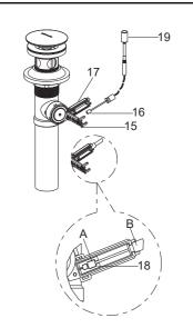
Open the coverplate(15) on the drain body, and insert cable end(16) into the square hole(18) of the cable box(17). Make sure the cable is properly buckled at both ends(A, B) of the cable box as the figure shown.
