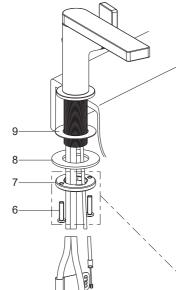
Position the faucet, install the screws(6) into the mounting nut(7).
