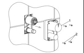
Remove the plastic guard(1) after completed the finished wall.
