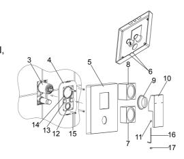
Install handle(10): Tighten the setscrew(11) with hex wrench(16). Press plug button(17) into the hole.
