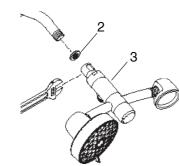
Put the washer(2) into the showerhead(3) and tighten the showerhead with a suitable wrench.
