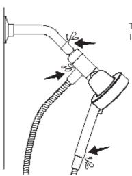
Turn on water supply and check all leakage.
