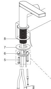
Position the faucet, install the screws(5) into the mounting nut(6).
