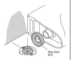
14 Carefully lower over brackets. 轻轻的将马桶降低,压在支架上。
