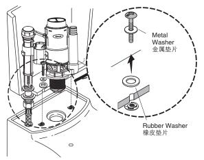
12 Thread the bolts into the bowl through the bolt holes in the bottom of the tank. Tighten the bolts using a screwdriver.
