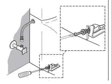
17 Connect supply and turn on the water. 连接供水管,打开水源。
