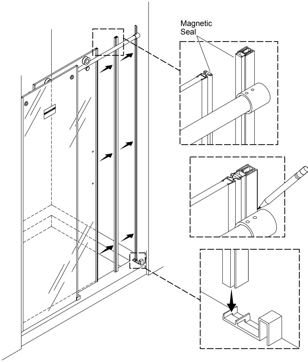
**NOTE:** The strike jamb must fit tightly against the threshold cap and the wall.
