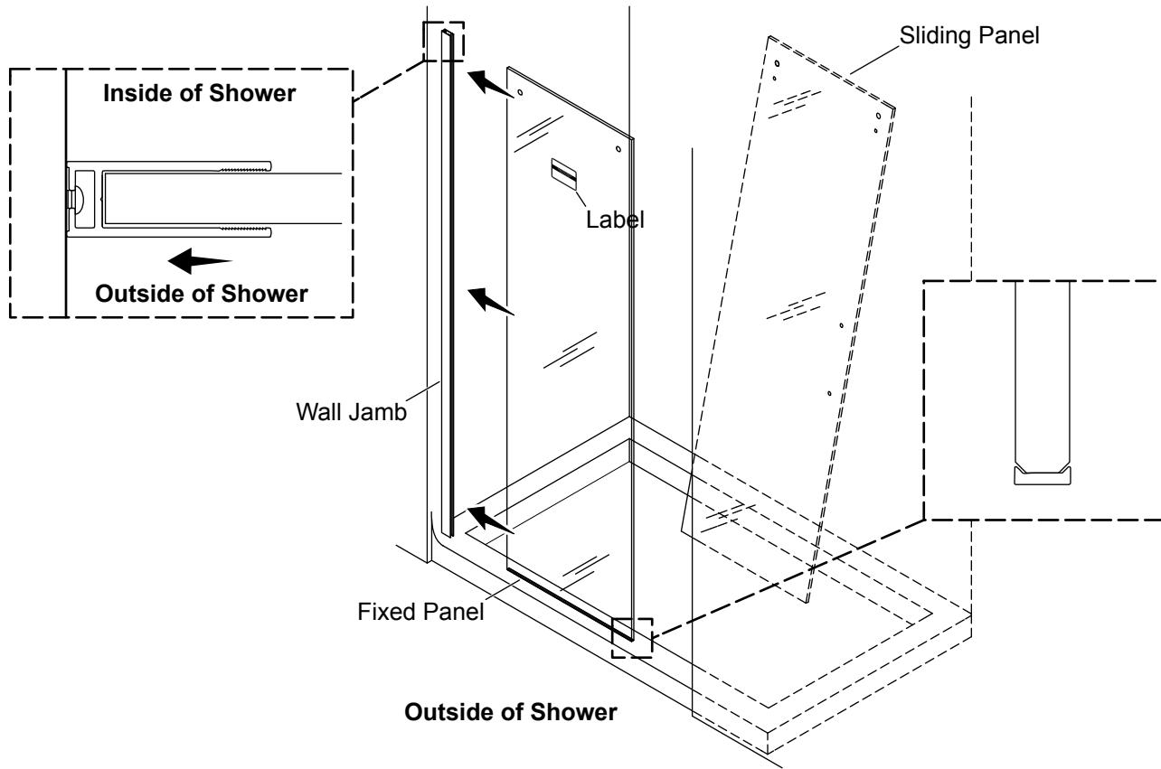
**⚠ WARNING:** The fixed panel is not secure in the wall jamb until the wedge seal and the header are installed. Use care until the installation is complete.
