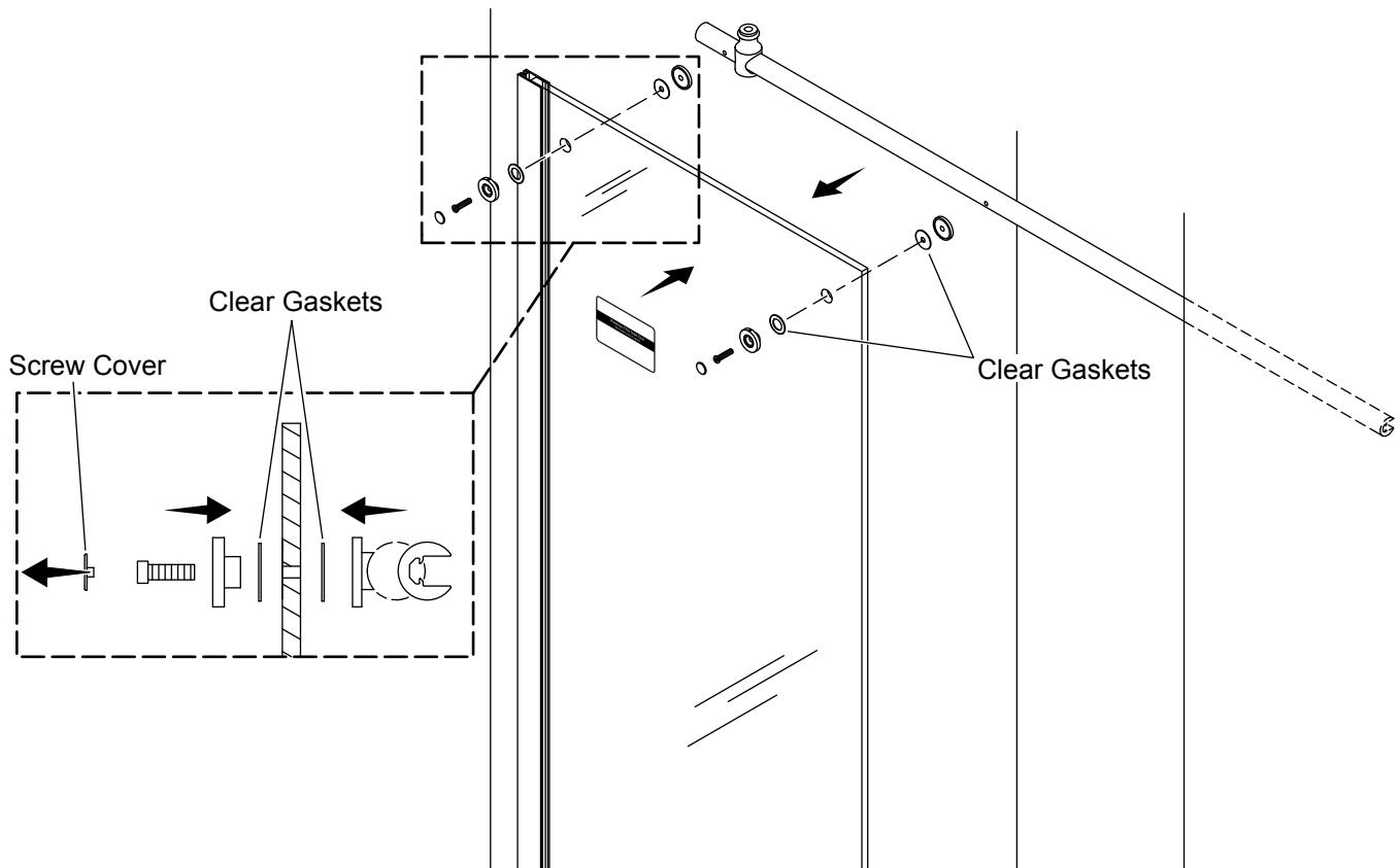
**IMPORTANT!** The header installs to the fixed panel on the inside of the shower.
