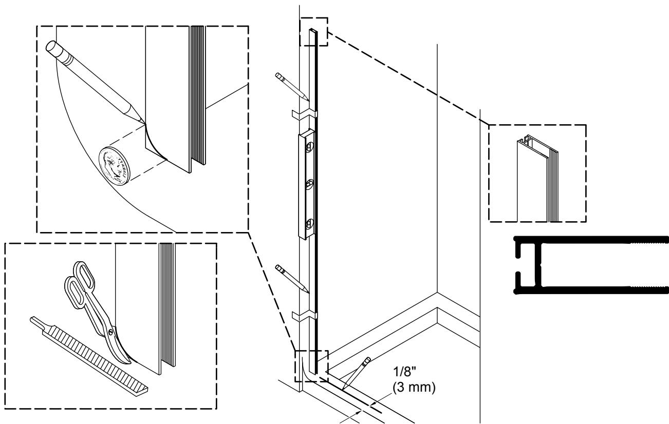
**IMPORTANT!** The wall jamb must fit tightly against the shower base and wall.
