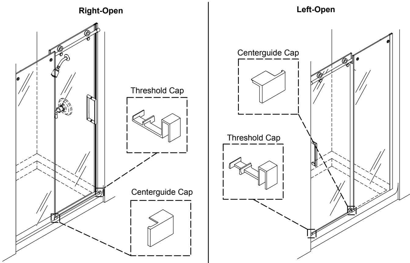
**IMPORTANT!** Right-Open configuration is shown in the installation steps unless otherwise indicated.
