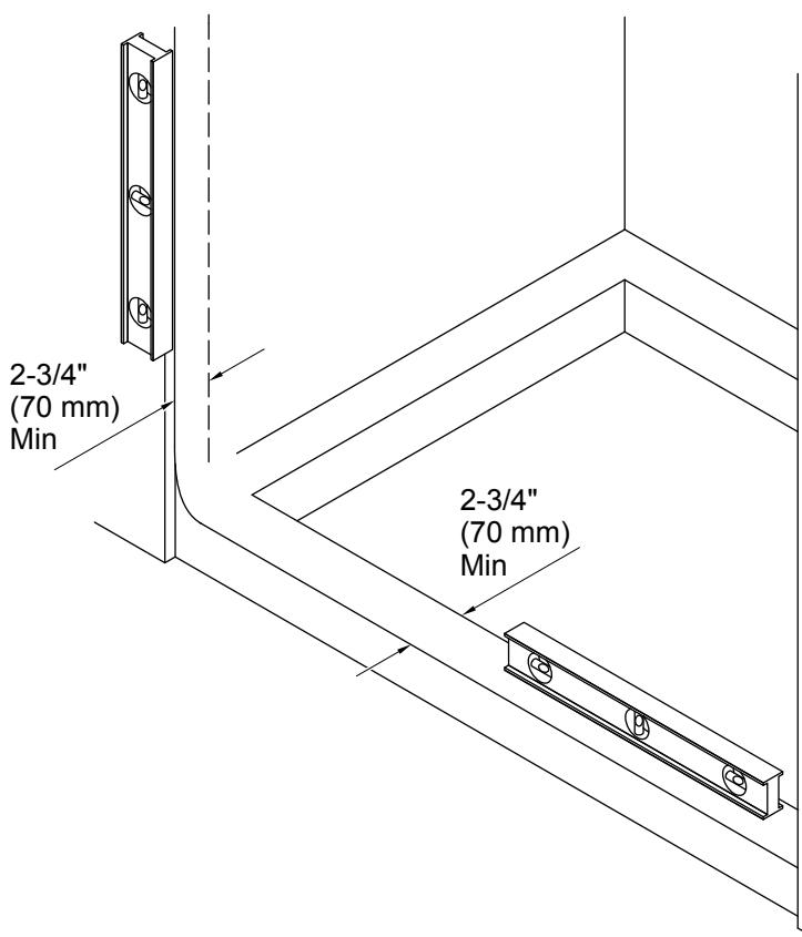
**IMPORTANT!** For proper door alignment and operation, confirm that the shower base and walls meet the following requirements. Do not install the door if these requirements are not met.
