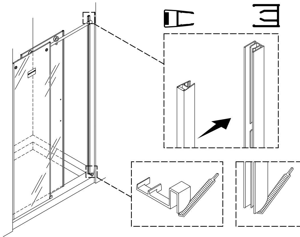
**NOTE:** The strike jamb must fit tightly against the threshold cap and the wall.
