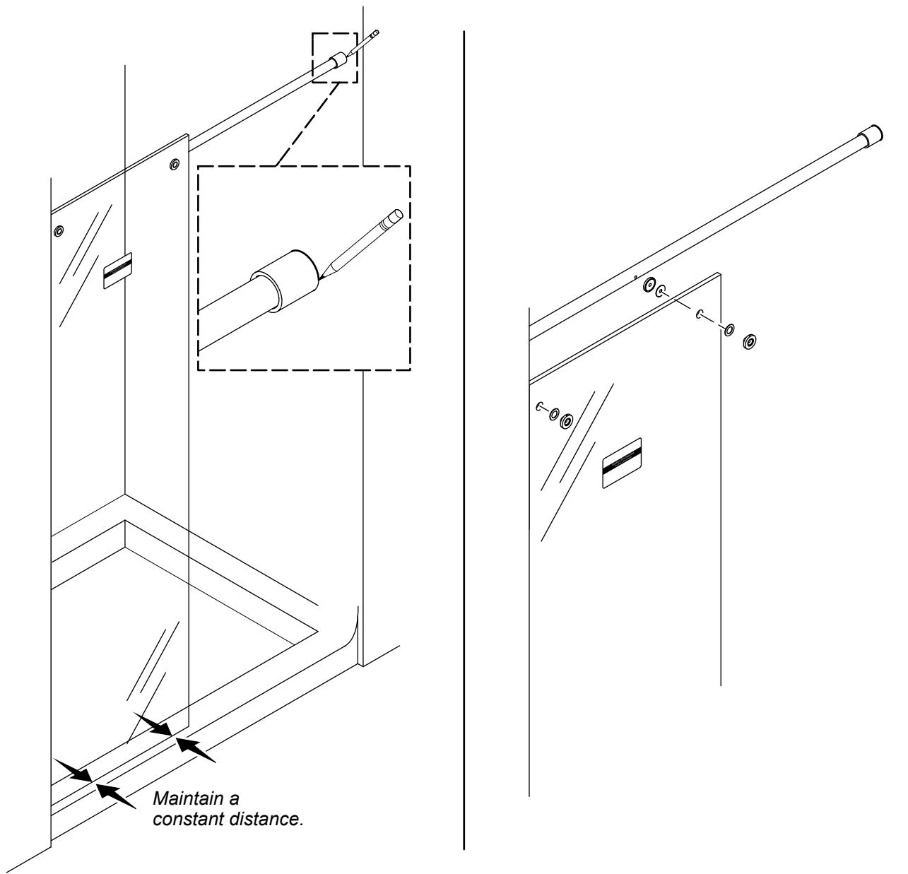
**NOTICE:** The header must be level and securely fastened to the fixed panel. If necessary, go back to the "Level the Header" section.
