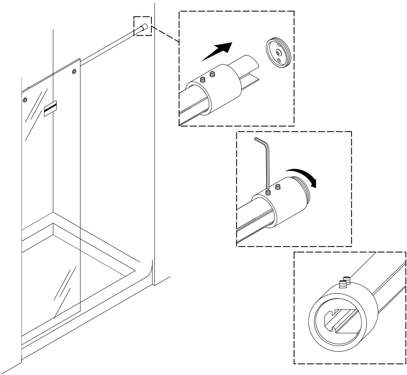
**IMPORTANT!** Do not use force to align the header with the wall bracket. If the header does not align, check that the header is level and the fixed wall panel is seated properly. If necessary, make small adjustments according to the "Level the Header" section.
