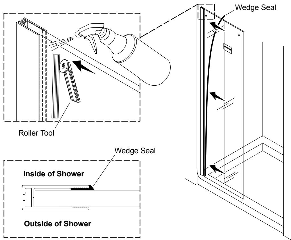
**⚠ WARNING: Risk of product damage.** Do not use sharp objects to push the wedge seal into place.
