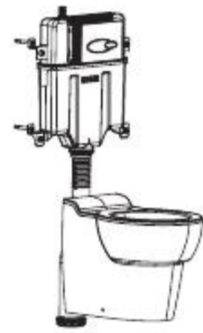
In-wall Tank Without Frame 入墙式隐藏水箱(不含固定支架)座便器
