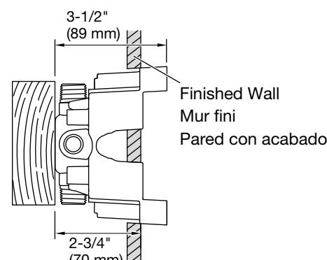
**6** Mount the valve body plumb using two #8 flathead screws.
