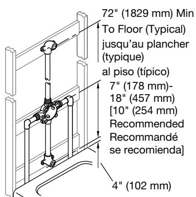
**NOTICE:** Use only 1/2" (5/8" OD) copper pipe (type L or M) between the valve and bath spout. Using other materials may cause water to flow from the showerhead and bath spout at the same time.
