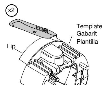
**Standard Models:** Cut a hole at the valve location. Mark the screw locations.
