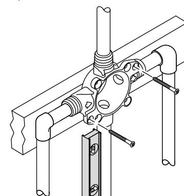
**7 Snap on the template (screws are not needed). Go to step 9.**
