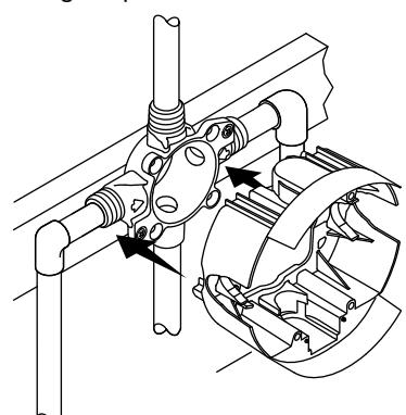
**8 Thin Wall Installations:** Cut the lip from the template with a utility knife or scissors.
