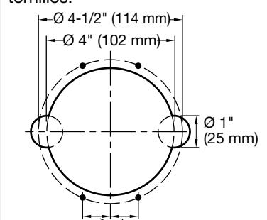
**Both Models:** Drill four 3/16" holes at the marked screw locations.
