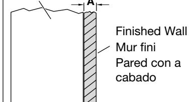
**5 Thick Wall Installations:** Mount the valve body support 2-3/4" (70mm) to 3-1/2" (89 mm) from the front of the finished wall.
