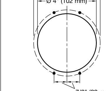
**Models with Stops:** Cut two holes for the stops. Cut a hole for the valve. Mark the screw locations.
