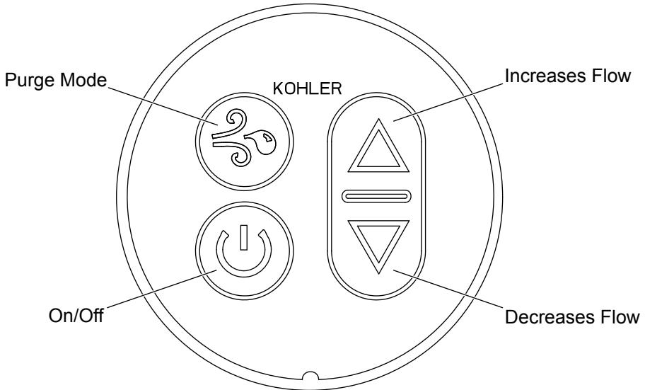
**IMPORTANT!** This product contains an automatic water purge mode that turns the blower on for 5 minutes after the unit is turned off and drained.
