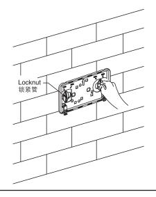
3. Pin the indentation on block screen with screwdriver to take out the block screen.
