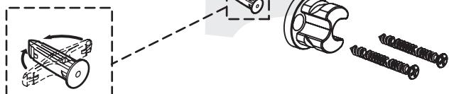
3. Fix the wall plate to the wall with screws.
