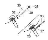
Fit the plastic washer (29), rubber washer (32), and retaining nut(28) onto the ball lever (30). Insert the ball lever assembly(33) into the drain lever hole (27) and through the stopper hole, and tighten the retaining nut. Be sure that the ball lever points to the back of the lavatory, tighten the locknut on the drain body. Remove any excess putty.
