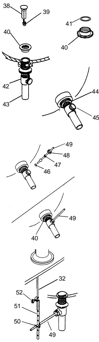
Apply thread tape to tailpiece(43) and install it to drain body(42). Insert drain body from underside of bidet with drain lever hole(45) facing to the back of the bidet. Thread flange(40) onto drain body by hand. Tighten the locknut(44) by hand from the underside.
