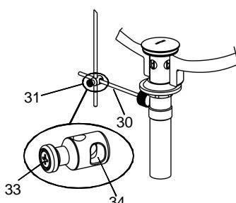
Insert the ball lever rod(30) into the bigger hole(34)
