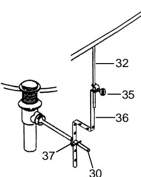
According to the lift rod length, bend the link(36).
