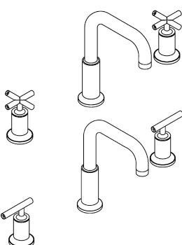
Insert the spout(16) to the shank until the bottom of it contacts the deck or bath tub. Tighten the screw(18) by hex wrench(17) provided, then insert the plug button(19) into rear hole.
