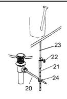
Assemble thumb screw(22) to link(21), and link onto ball lever rod(20) with "V"-clip(24). Slide lift rod(23) through hole in faucet and into the hole in link. Position the lift rod (Push the ball lever down into the open position, and adjust the lever to make sure the height between lift rod and table is controled within the range of 70~75mm). Tighten thumb screw.
