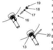
Place the rubber washer(16) into the drain lever hole. Put another plastic washer(17) and retaining nut (18) into the long end of ball lever rod(19). Insert the ball lever assembly(20) into the drain lever hole and through the stopper hole, and tighten the retaining nut(18).
