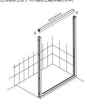
Install the door glass. Note: The external door glass should be hung from the inside to the outside and the internal door glass should be hung from the outside to the inside. Both should be carried out at the inner side of the rail.
