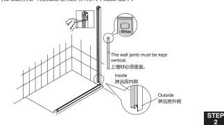
Fix the wall jambs. Snap two jambs into the bottom rail from the top and then fix them onto
