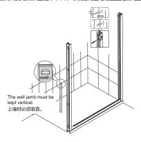
Install the top rail. Snap the top rail into the top of the wall jambs and adjust it level. 安装上导轨。将上导轨从上往下卡入墙材上端,并调好水平。
