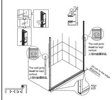
Make sure the ceiling is firm enough and then fix the top frame onto the ceiling. 将顶横梁固定在天花板上。之前请确定天花板是足够的牢固。
