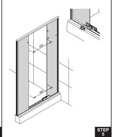
Lift the door glass and insert into the bottom hinge. 将门玻璃拾起,插入下铰链里。 IMPORTANT: When the door glass is closed, first
