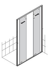
Install the bottom hinges onto the glass panels. Adjust the distance between the panel glasses to about 680 mm. 安装下铰链到固玻,之后调节固玻之间的尺寸,约为680mm。
