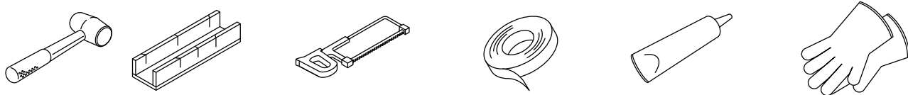
Rubber Mallet Miter Box 32-Teeth Per Inch Blade Masking Tape 100% Silicone Sealant Protective Gloves
