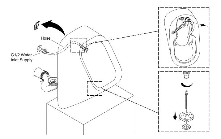
**IMPORTANT!** To avoid damaging the strainer, remove the strainer when cleaning the urinal with abrasive cleaning materials or scouring pads.
