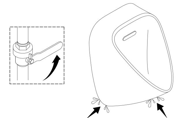
**NOTE:** If water splashes or overflows when the urinal is flushed, adjust the water pressure lower using the control stop.
