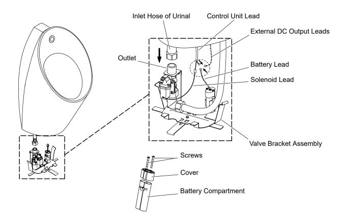
NOTE: Verify that the batteries polarity is correct. Do not mix old and new batteries.
