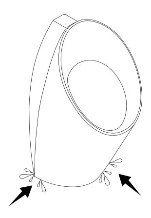
NOTE: If water splashes or overflows when the urinal is flushed, adjust the water pressure lower using the control stop.
